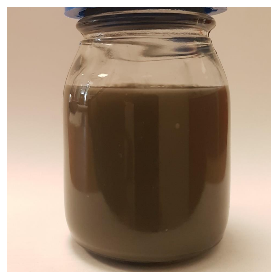
Image of silver Nanocolloid with PVP (SNP514)
