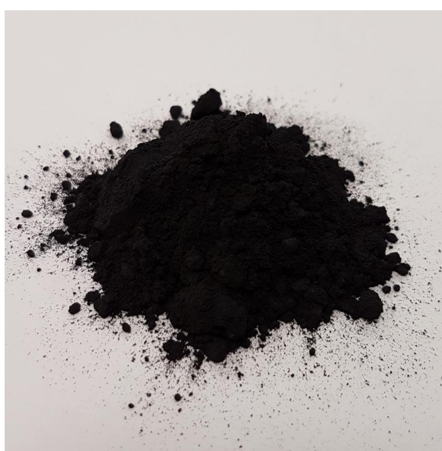
Image of graphene nanoplatelets (GP7)
