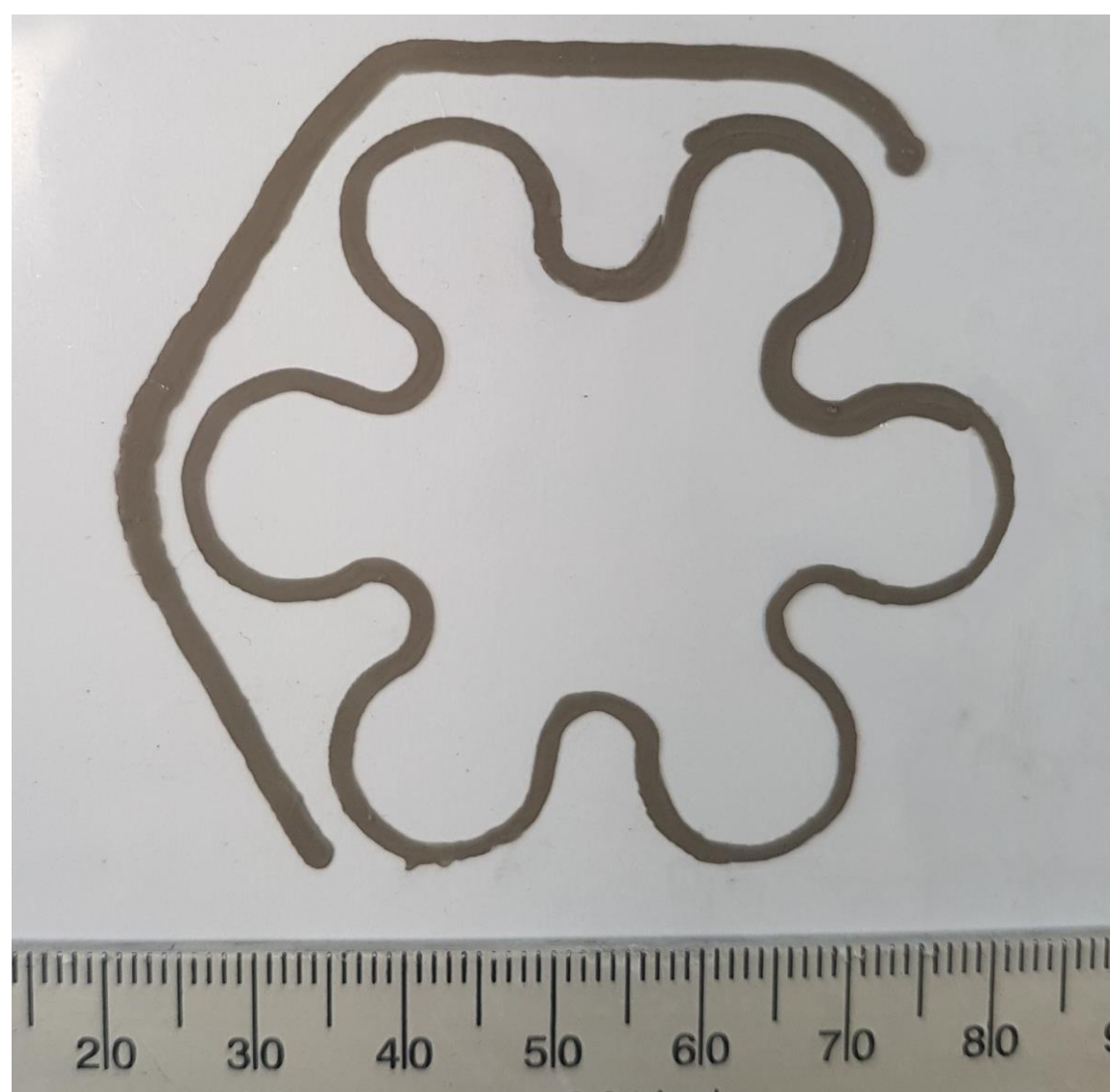
Printability of ARMINK-S1 with 3D printer (800 \mu\text{m} nozzle)
