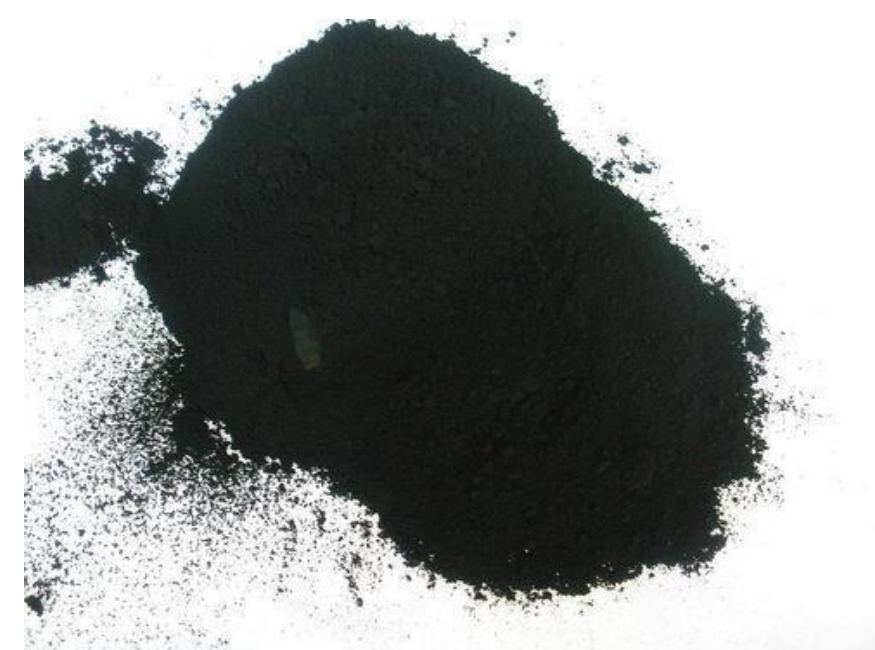
Image of zero-valent iron nanopowder (FNP201)
